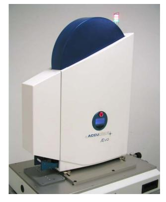
• The bench top configuration consisting of a base with feet, built-in power supply, and 2-hand control provides a simple cost-effective solution.
