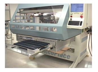
The optional vision system ensures an accurate assembly by scanning both the mesh and the target part prior to placement.
