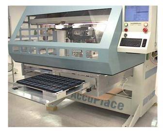
along with AccuPlace's patented peeling technology ensures that the adhesive parts are peeled and placed accurately onto the target part.
