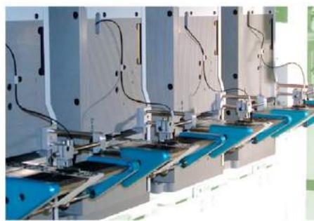
Up to four robot models RM3065 can be integrated into the APAC. This allows feeding of up to 4 different adhesive components, allowing the execution of complex assembly tasks.
