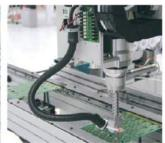
Assembly of adhesive backed dome switch arrays onto a PCB. PCB shows very high tolerance.
