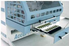
To load/unload the APAC, various transport systems such as dual tray shuttle, SMEMA conveyor, or tray handling units can be integrated.
